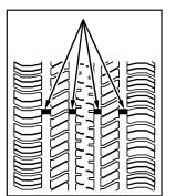
One way to tell when it is time for new tires is to check the treadwear indicators, which will appear when your tires have only 1/16 inch (1.6 mm) or less of tread remaining. You need new tires if any of the following statements are true:
